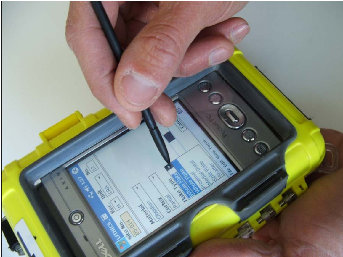
Figure 1. Dell Axim PPC used inside weatherproof Otterbox container for recording site, artifact, feature, shovel test, and landscape details directly to project databases.
