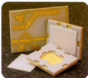
Point-to-multipoint transceiver for 24.5 to 26.5 GHz (Source: IMST, Germany)
