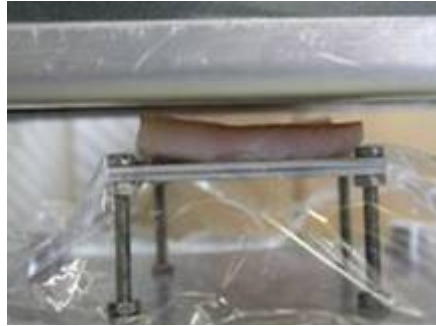
Figure 3: View of a swine skin sample being measured for radioactive contamination using an ADM-300C with the ABP 100 attachment.
