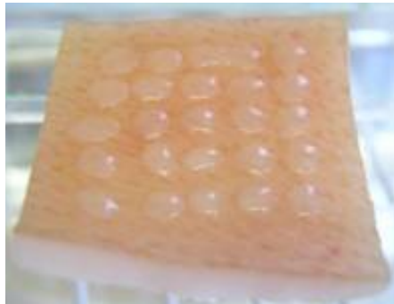
Figure 1: A swine skin coupon spotted in a 5x5 grid with an aqueous radionuclide.
