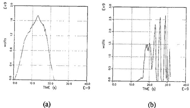
**Figure 6** Electron beam power (a) injected into the plasma-filled transport tube, and (b) after 3.4 m of propagation in the plasma-filled transport tube.
