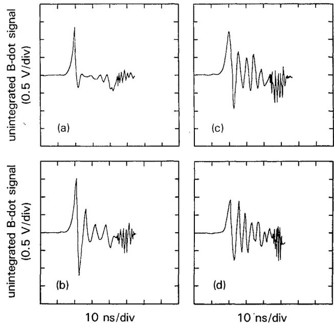
**Figure 3** Unintegrated B-dot loop response 0.9 m downstream from the entrance to the plasma filled transport chamber; (a)  $n_p=0$ , (b)  $n_p=6.3 \times 10^8$  cm<sup>-3</sup>, (c)  $n_p=1.0 \times 10^9$  cm<sup>-3</sup>, (d)  $n_p=1.5 \times 10^9$  cm<sup>-3</sup>.
