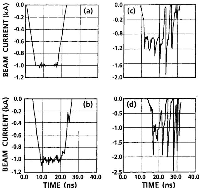
**Figure 5** Beam current waveforms from the MAGIC simulation at (a)  $z=0 \text{ m}$ , (b)  $z=1.1 \text{ m}$ , (c)  $z=2.3 \text{ m}$ , and (d)  $z=3.4 \text{ m}$  downstream from the entrance to the plasma filled transport chamber for  $n_p = 2.0 \times 10^9 \text{ cm}^{-3}$ .
