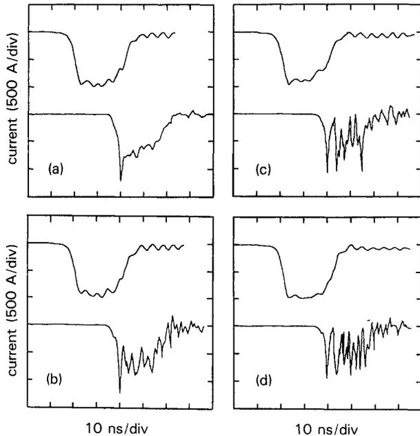
**Figure 2** Current waveforms from the resistive wall current monitors; (a)  $n_p=0$ , (b)  $n_p=1.0 \times 10^9$  cm<sup>-3</sup>, (c)  $n_p=1.5 \times 10^9$  cm<sup>-3</sup>, (d)  $n_p=2.0 \times 10^9$  cm<sup>-3</sup>. Top (bottom) waveform: current entering (exiting) the transport chamber.
