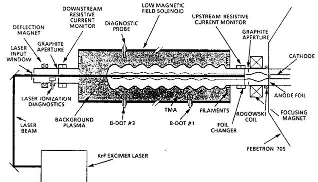
Figure 1 Schematic of the plasma wakefield experiment.
