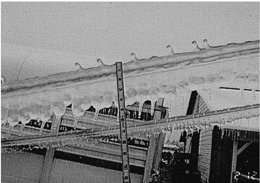
Fig. 2. Freezing rain ice accretion in Arkansas, February 1994 (photo Entergy).
