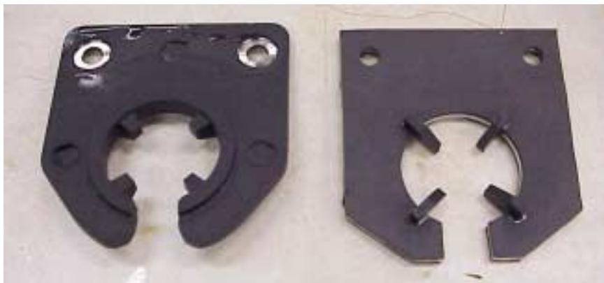
**FIG. 5. Comparisons of the original and the redesigned sensor mounting brackets.**
