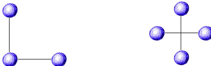
FIG. 2. Two configurations for measuring the gradient in two dimensions. For the arrangement on the left, the phase centers of the two dipoles and of the equivalent pressure formed by summing all three elements are not coincident. In contrast, the phase centers for both dipoles and the equivalent pressure for the arrangement on the right are coincident. The four-sensor arrangement has zero in-plane phase error.
