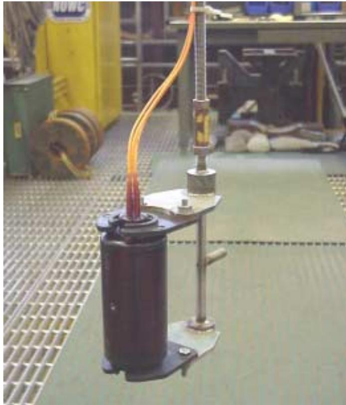
**FIG. 1. Vector sensor (Wilcox Research Prototype 01).**
