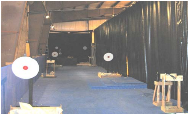
Figure 1: Experimental approach arena, with shooting stations, targets, and marksman's station (threat source) at the far end
