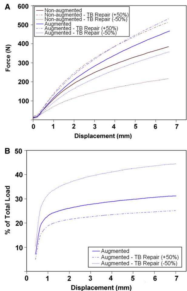
**Figure 2** Parametric variation in parameter *A* of the tendon-to-bone (TB) repair (spring #1). (A) The biomechanical performance of the nonaugmented and augmented repair constructs and (B) the percent load carried by the scaffold augmentation component for simulated tendon-to-bone repair.
