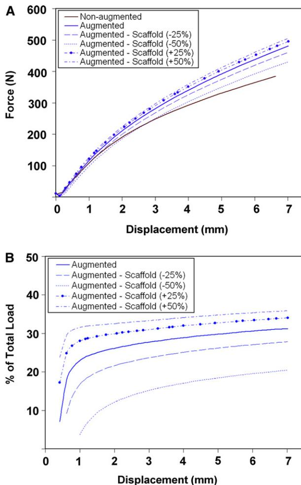
**Figure 3** Parametric variation in parameter A of the scaffold augmentation component (spring #3). (A) The biomechanical performance of the augmented repair construct and (B) the percent load carried by the scaffold augmentation component for simulated scaffold augmentation component.
