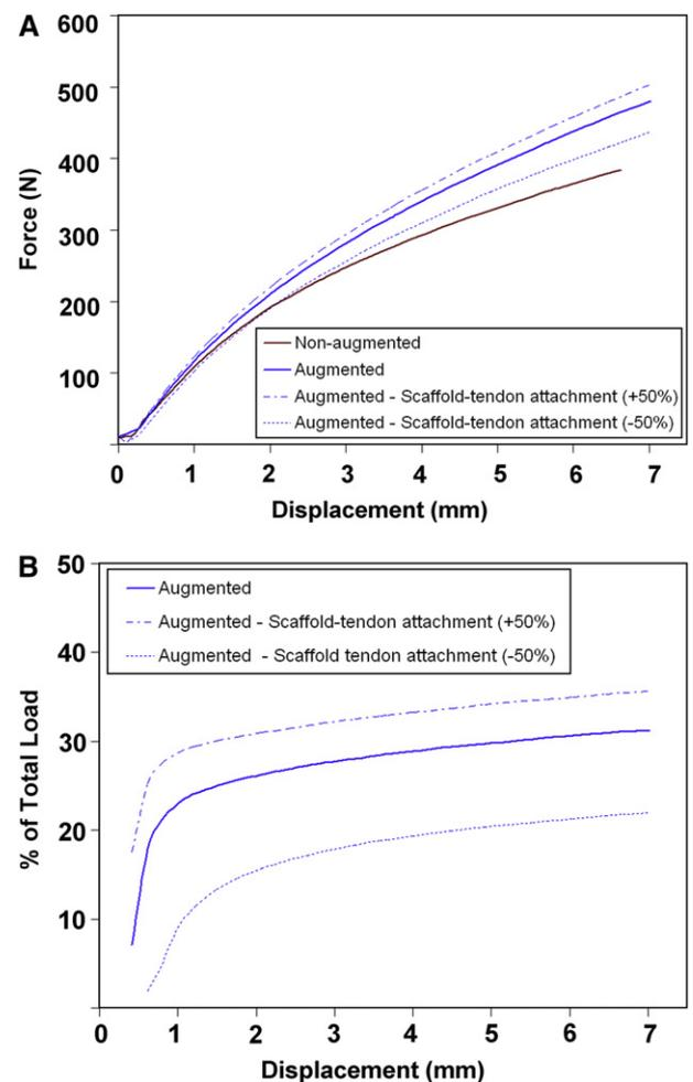
**Figure 4** Parametric variation in parameter A of the scaffold-tendon attachment (spring 4). (A) The biomechanical performance of the augmented repair construct and (B) the percent load carried by the scaffold augmentation component for simulated scaffold-tendon attachment.
