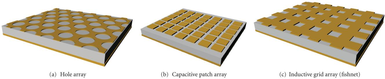
FIGURE 13: Designs less sensitive to polarization effects.
