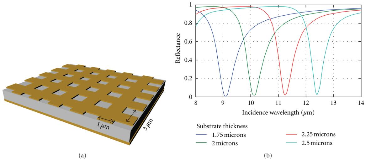
FIGURE 14: RCW simulations for inductive grid array shown in Figure 11(c). Here as the substrate, assumed to be ZnSe, is varied from 1.75 to 2.5  $\mu\text{m}$ . The resonant absorption wavelength shifts to longer wavelengths; however, the magnitude of the absorption remains near perfect.
