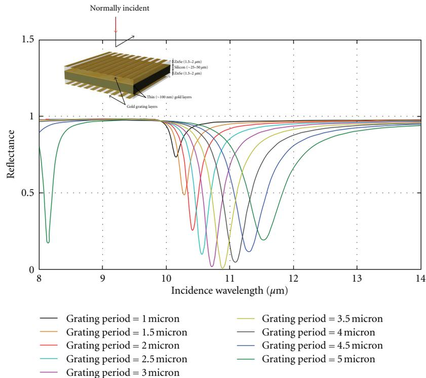
FIGURE 5: Simulation results, using the RCW method, that present the reflectance at normal incidence within the LWIR band as the gold grating period is varied from 1.0 to 5.0  $\mu\text{m}$ . For this simulation, the substrate thickness is fixed at 2.0  $\mu\text{m}$  with a grating duty cycle of 50%. The incident wave was normally incident with parallel polarization.
