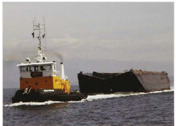
A bottom-opening barge containing drift debris being towed out to sea for ocean disposal
