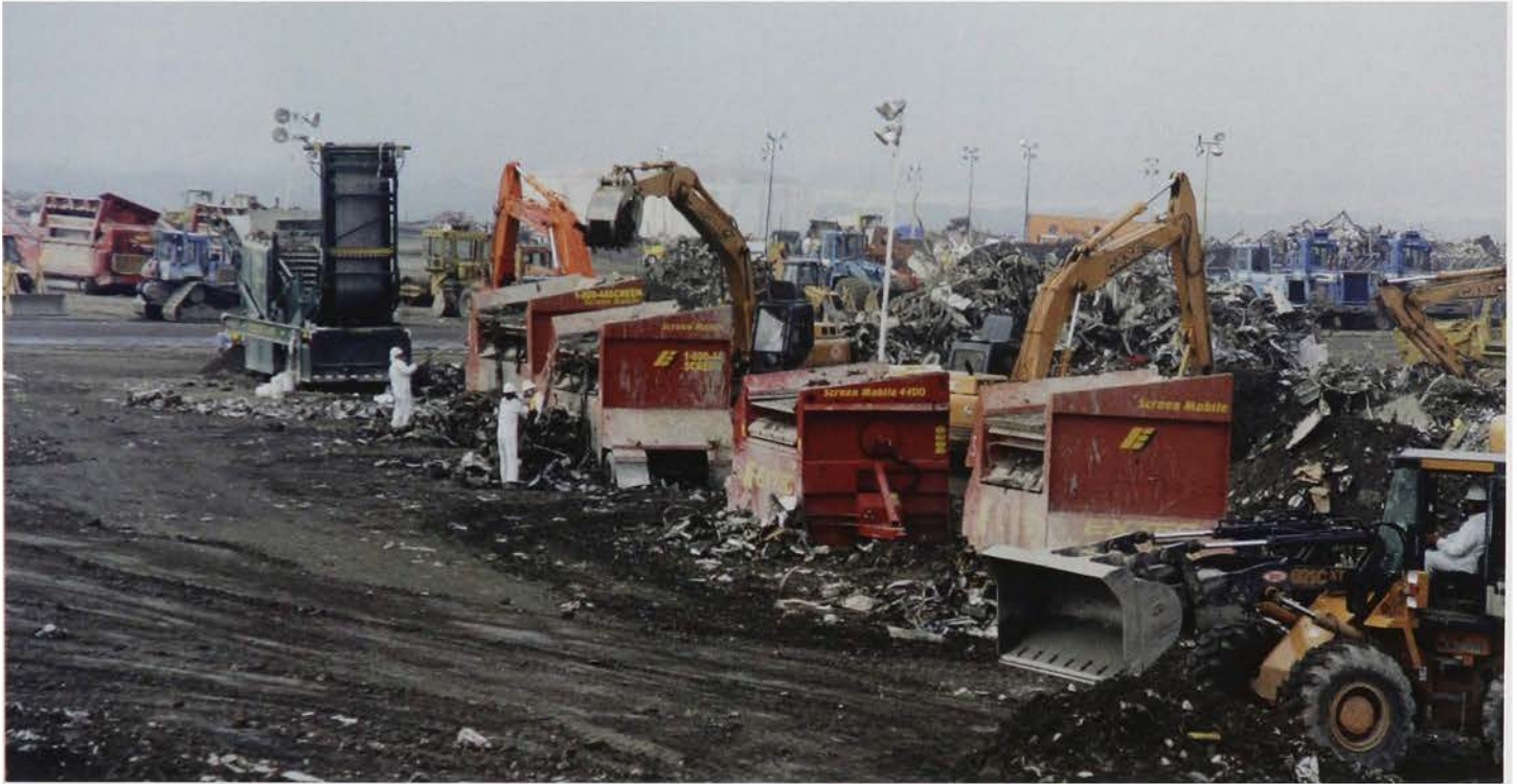
Backhoes load debris into sifters at the Fresh Kills landfill on Staten Island
