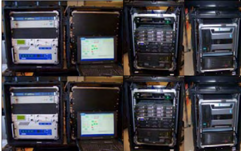
Figure 20. Commercial Common Imagery Processor in Four Transit Cases (from Jank, 2011)
