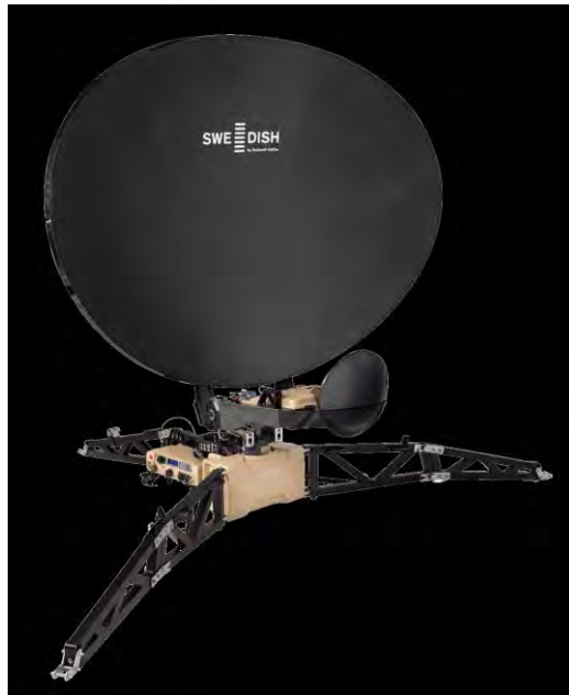
Figure 21. Rockwell Collins SWE-DISH CCT200 (from Rockwell Collins, 2012)
