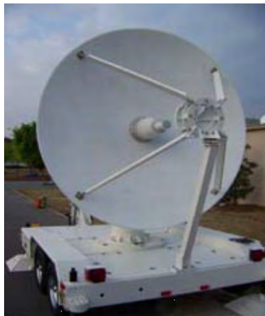
Figure 19. Remote Ground Terminal Downlink Dish (from Jank, 2011)
