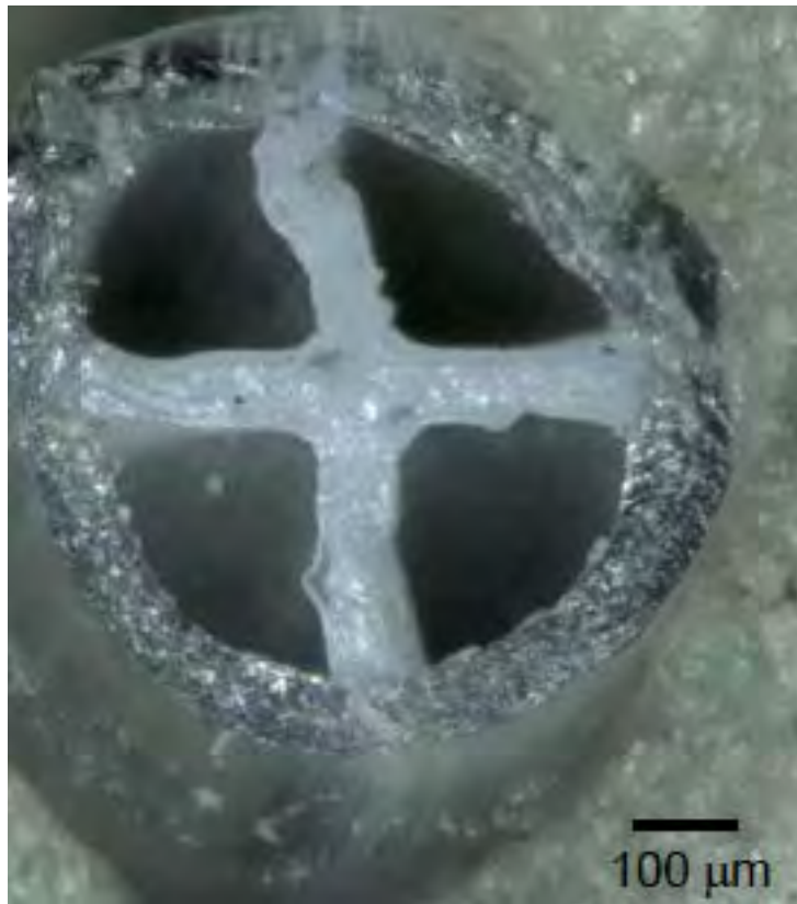
Figure 5. Magnified image of FDM filament showing internal gaps (from Holmes, 2014)
