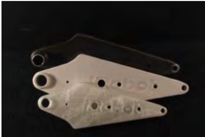
Figure 7. Printed lightweight flippers for PackBot (from Zunino, 2014)
