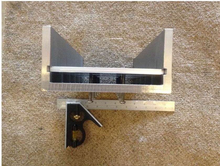
Figure 13. Photograph of stainless steel 4-point bending rig used to apply elastic stress to aluminum plate samples, from [8].
