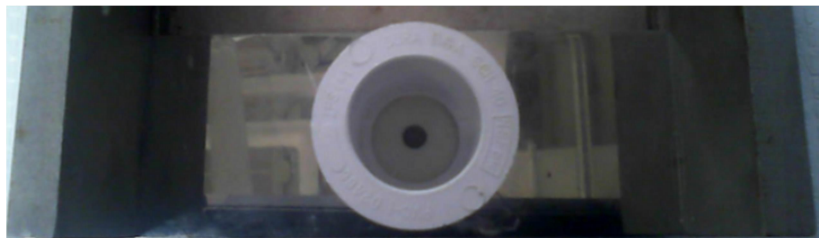
Figure 15. Top view of cup mounted to top of sample with double-sided tape. The area exposed to saltwater is punched through the tape.
