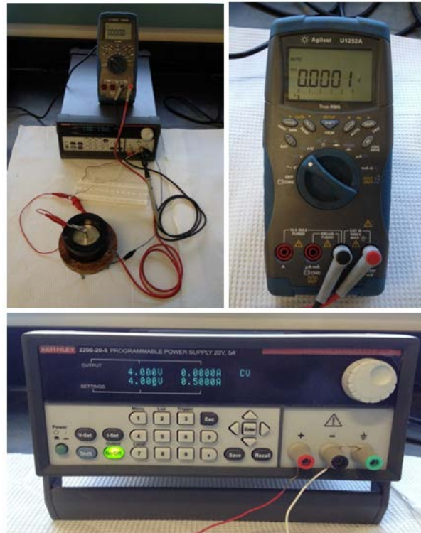
Figure 10. Setup to measure voltage across capacitor
