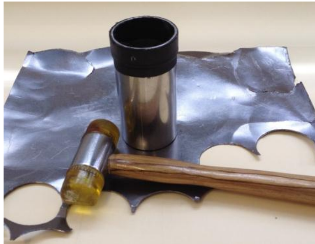
Figure 12. Die and hammer utilized in cutting Grafoil disk
