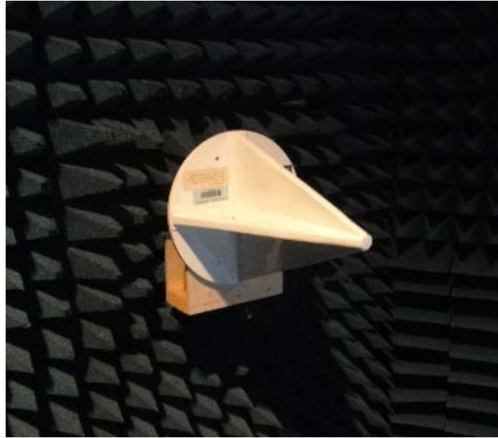
Figure 4. Transmission Antenna (Tecom 201302) Used for Emission of Test Signal
