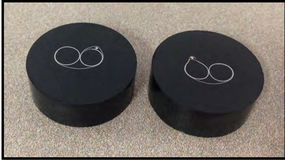
Figure 19. Phenolic pucks containing RES-treated substrates.
