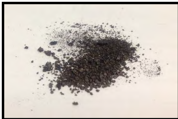
Figure 28. Black powder particles remaining in the alumina boat following treatment of the brass substrate.
