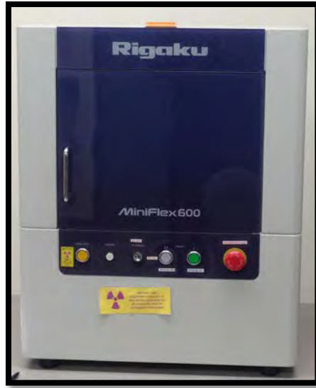
Figure 24. Rigaku MiniFlex 600 used for X-ray diffraction.
