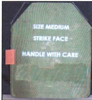
Figure 10. Hard Armor Plate with Rubber Edge Strip
