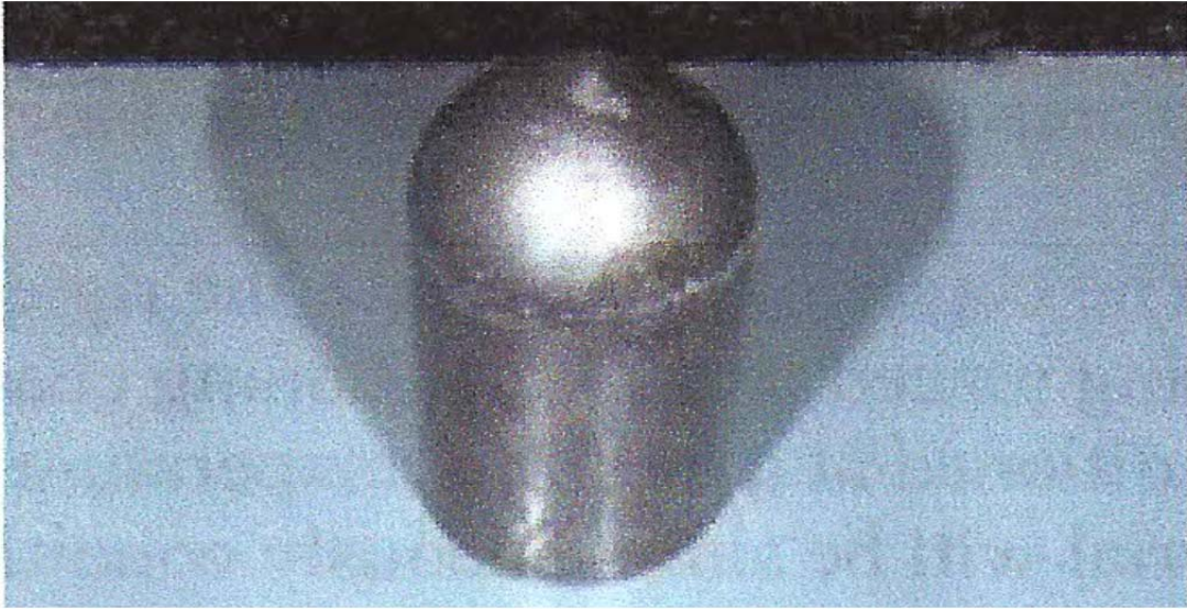
Figure 4. Cylindrical Steel Mass Used for Drop Tests on Clay
