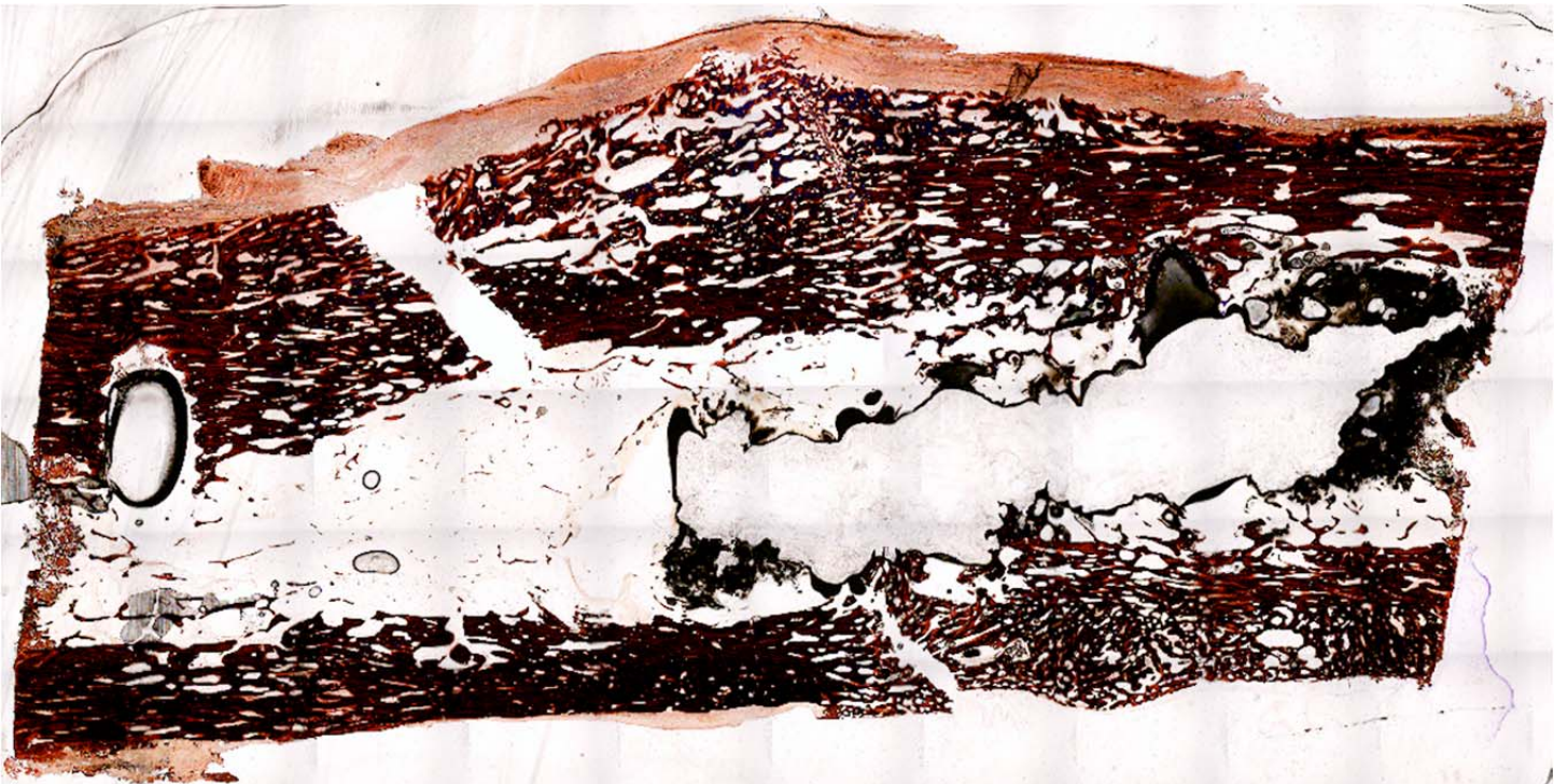
Figure 92: Hard sectioning histology image of Segmental Defect Dog 5 implanted with canine cadaveric allograft, stained by Masson's Trichrome method. Overview of mid-diaphysis of right tibia with canine cadaveric allograft. The black tissues in the middle level at right half are the bone marrow soft tissues. The oblique crack was the fracture generated by biomechanical testing.
