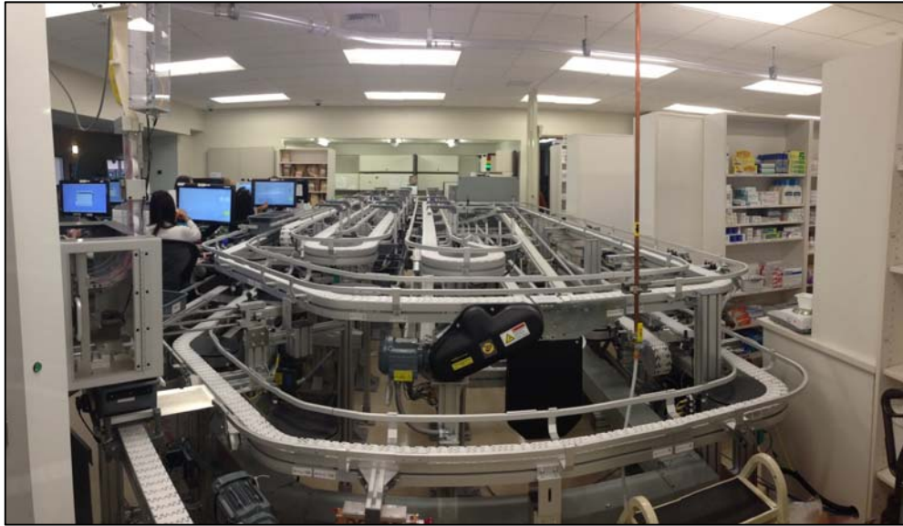
Figure 2. Conveyer Belt Installed at Naval Medical Center San Diego. Once the customer places an order, the conveyer system directs each prescription through the different steps of the fill process. Manual fill stations are located to the right side of the conveyer belt; as pharmacy technicians complete a manual fill, they place completed orders onto the conveyer belt for routing to pharmacist verification.
