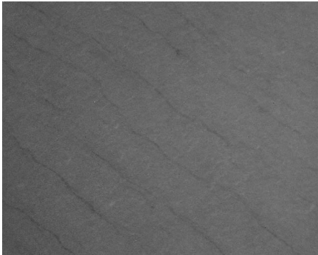
Figure 4. (a) Example of fine-scale IR imagery as observed from the aircraft under moderate wind speed. Each image is roughly 160 m x 200 m, the top of the images is East, and the wind is from the NE. (b) Temperature and its derivative measured along the flight track that correspond to the observations in (a).
