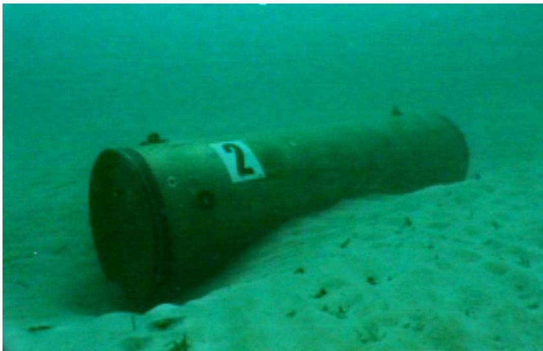
Figure 2 – Partially Buried Instrumented Mine in Fine Sands. Scour developing on ends.
