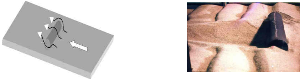
Figure 2 (left): A schematic showing the formation of energetic horseshoe tip vortices at the lee side of a cylinder during the onshore water motion (large arrow).
