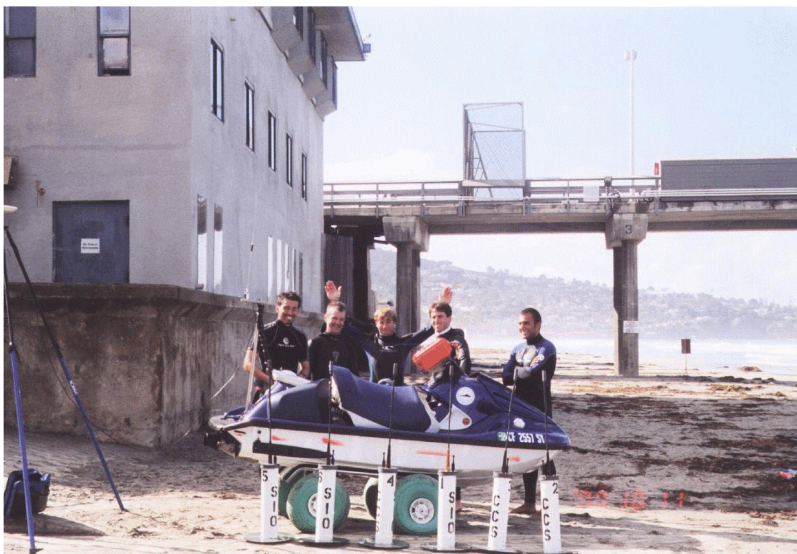
Figure 4. [Photograph of 6 surfzone drifters on the beach near the Scripps pier. The 50 cm tall drifters contain GPS, and transmit their position to shore in real time, and also record their trajectories internally.]
