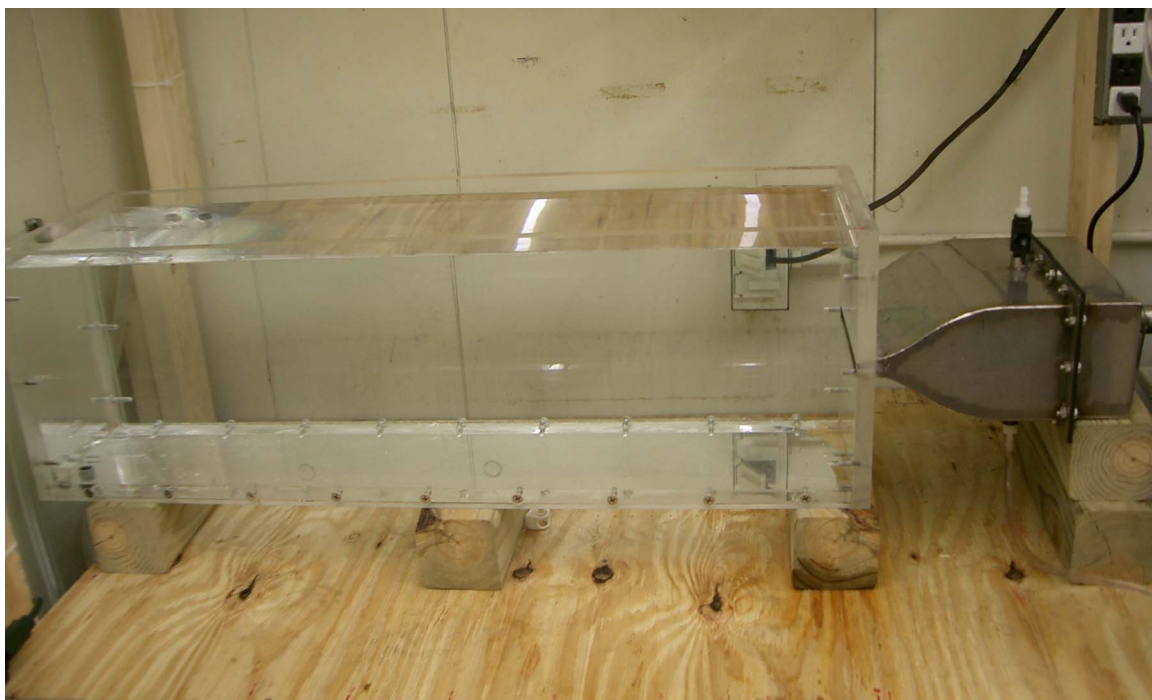
Figure 1. Photograph of new flume located in the temperature-controlled room.
