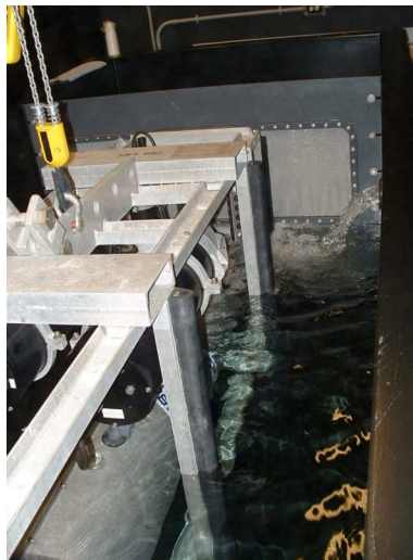
Figure 1. HIDEX II being readied for calibration in the 2500-gallon test tank in the newly completed Marine Biophotonics Center. The HIDEX II is supported by the articulating crane and the inlet is coupled to a filtration baffle that insures that none of the bioluminescent dinoflagellates used in the biological calibrations are recycled through the detection chamber.
