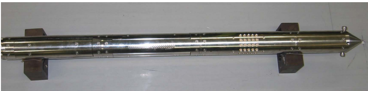
Figure 1 In-situ probe composed of three effective earth pressure transducers, a dynamic pore pressure transducer and a tide gage.
