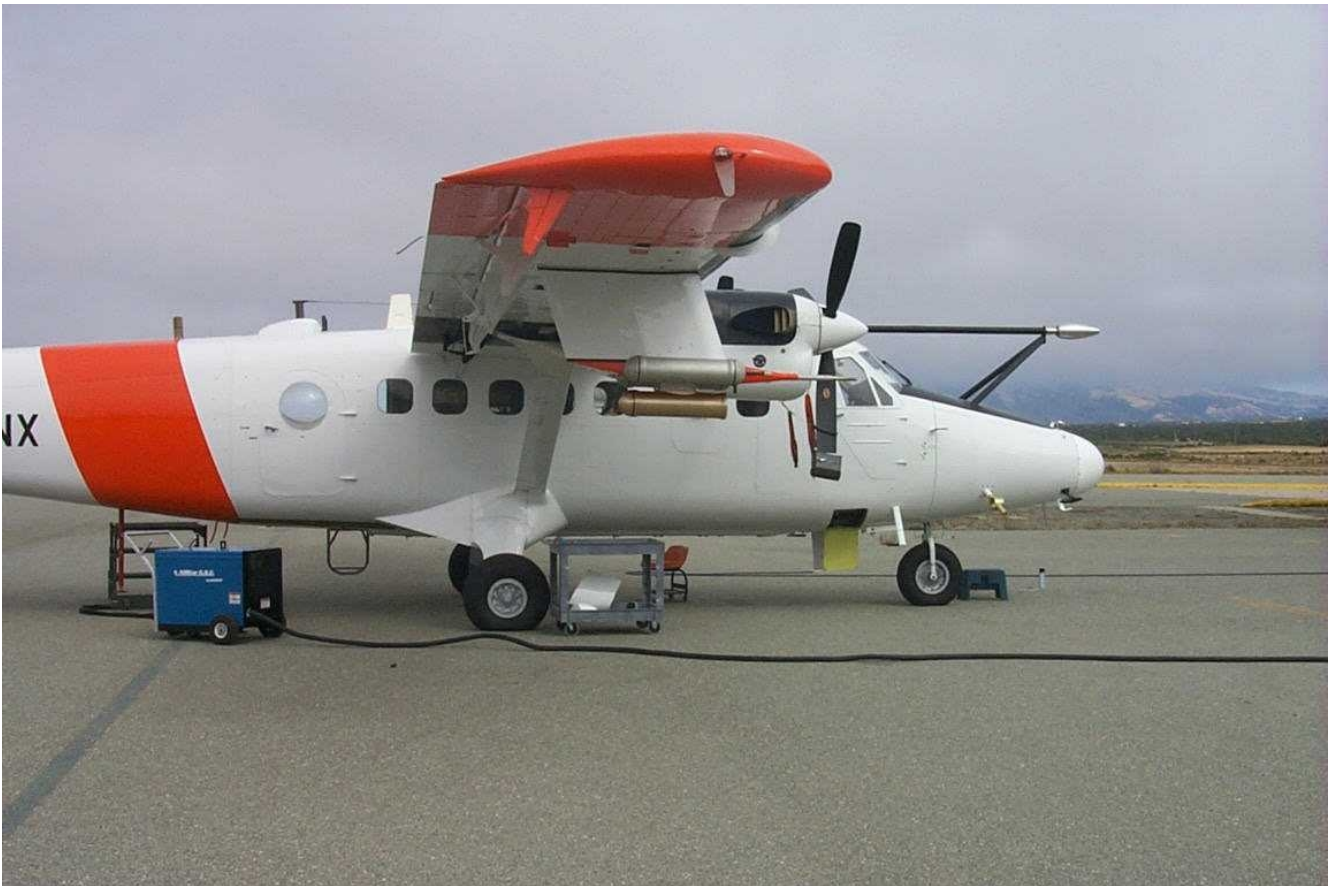
Figure 1: CIRPAS Twin Otter Research Aircraft. Turbulence and auxiliary sensors are located in and around the radome.
