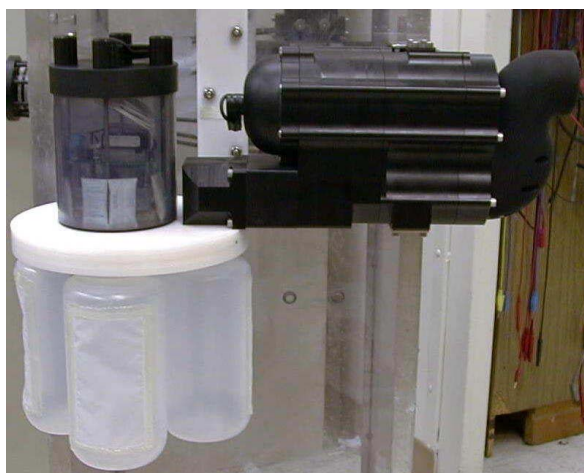
Figure 2: Generation 3 MBBP with attached plankton catcher on the instrument outflow.
