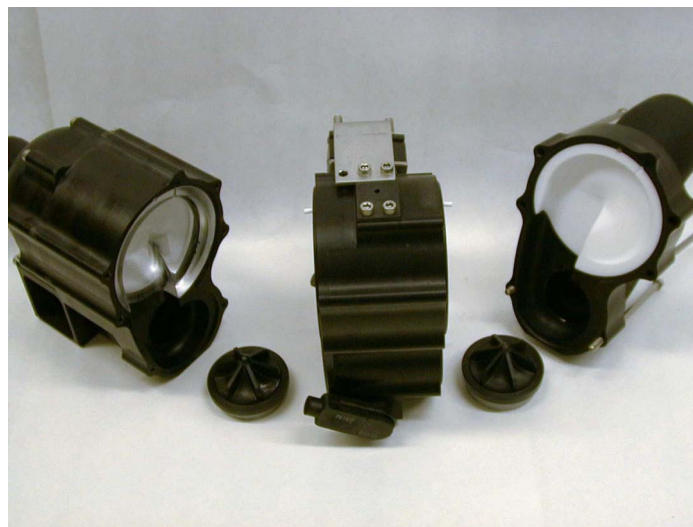
Figure 1: The 3 sections of the Generation 3 MBBP, with impeller and flow meter actuators.
