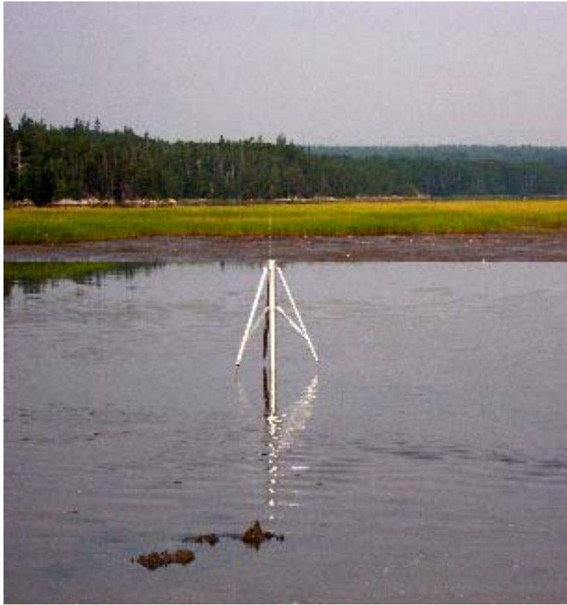
Figure 1: Sediment lander deployed at our field site in Cole Harbor, Nova Scotia. The lander is fitted with probes to measure temperature and the critical stress intensity factor, K_{Ic}
