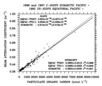
Figure 2. Comparison of POC determined from MULVFS samples vs. simultaneously measured beam attenuation coefficient, *c*. The two dashed lines are the least sqares fit to data from two 2600 km NS transects at 140W in the equatorial Pacific. The solid line fits seasonal sampling along EW "line P" at 50N between the continental margin and ocean station PAPA (50N 145W).
