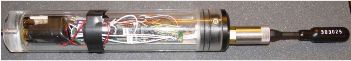
Figure 1. One of six autonomous recorders based on bioacoustic probe design of Bill Burgess of Greeneridge Sciences, Inc. Note the presence of 4 AA batteries, which provides sufficient power to fill 1 Gb of memory at various sampling rates. The package also includes a inclinometer, pressure and temperature sensors. The HTI hydrophone is detachable to permit a shore-power connection.
