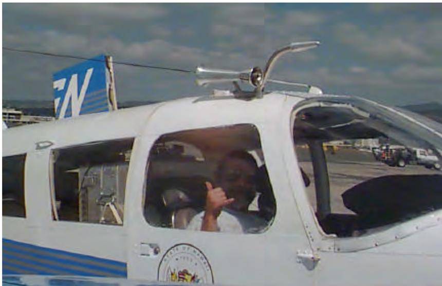
*Fig. 2. Aerosol inlet, venturi and temperature/humidity sensors are mounted atop Seneca passenger door. Aerosol instrument package is visible behind the passenger seat.*
