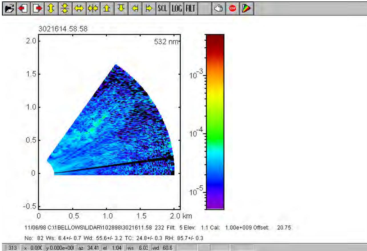
**Fig. 8** This horizontal lidar scan at about 10 m reveals the patchy structure of aerosol plumes from the offshore breaking waves (Fig. 1b) and which give rise to the patchy structures shown in Fig. 7 near the tower top.
