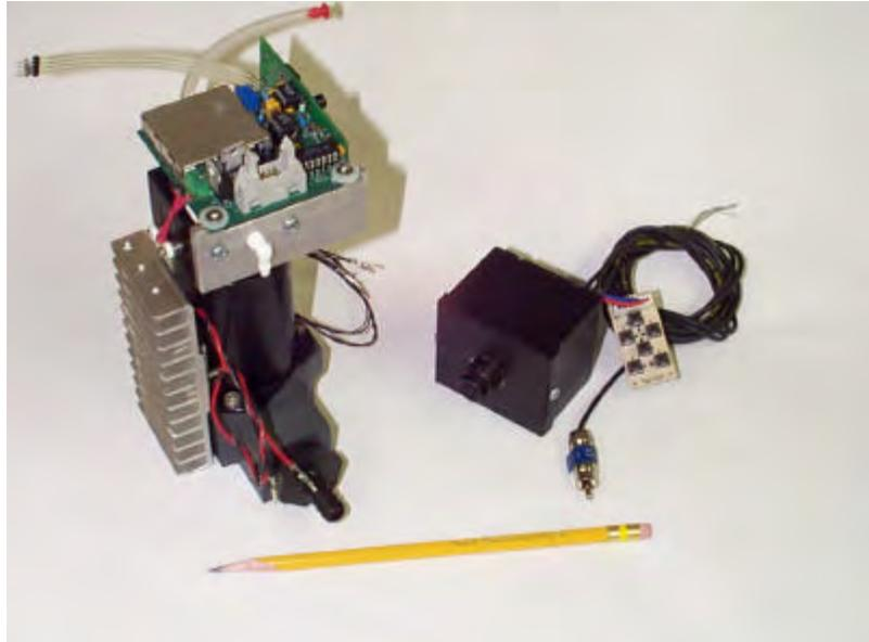
*Fig.5 Our 2.2lb stripped TSI 3010 counter (detector courtesy of TSI) on left and showing NASA pulse counter card (courtesy Dr. Chuck Brock) and cooling fins that will extend through fuselage. On right is our TV quality color video camera with annotation keypad.*
