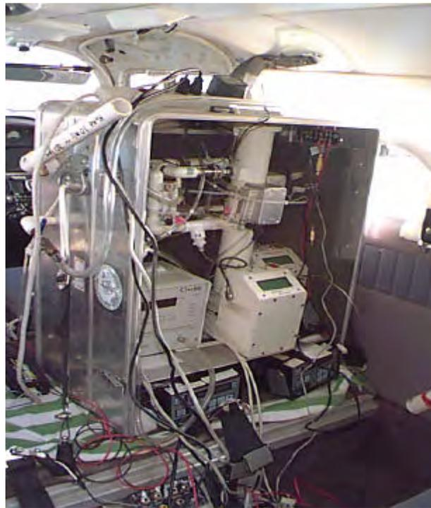
*Fig. 4 View of aerosol package during installation with inlet plumbing to two nephelometers to right of box, CN counters to their left and Met 1 particle counters below. Datalogger, GPS and microcomputer attach in front of box for operator use after installation is complete. An external forward scattering spectrometer probe (FSSP-300x) is mounted below the fuselage and provides ambient size distributions (0.3-20 $\mu$ m or an optional 0.5-40nm).*
