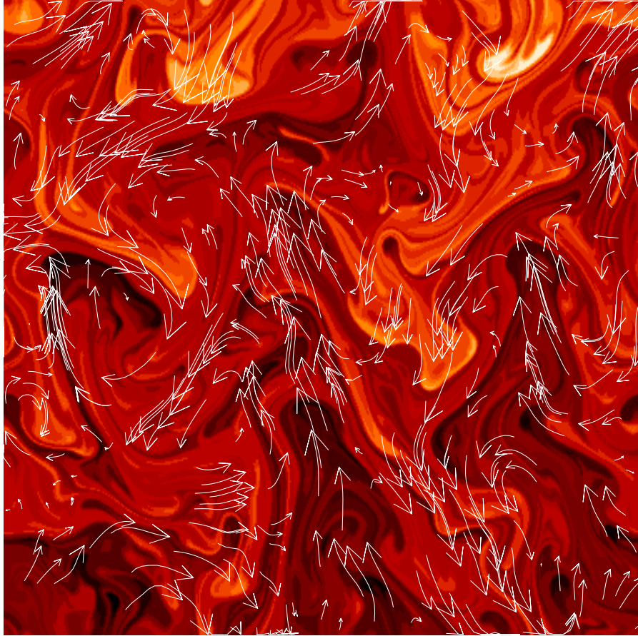
Figure 2: Two-dimensional salt fingering in seawater at buoyancy ratio R_\rho = 1.25 , from a 1024 \times 1024 numerical simulation. Lighter shades indicate higher concentrations of salt, and dark shades lower concentrations; velocity is indicated by arrows. The domain is approximately 16 cm wide.
