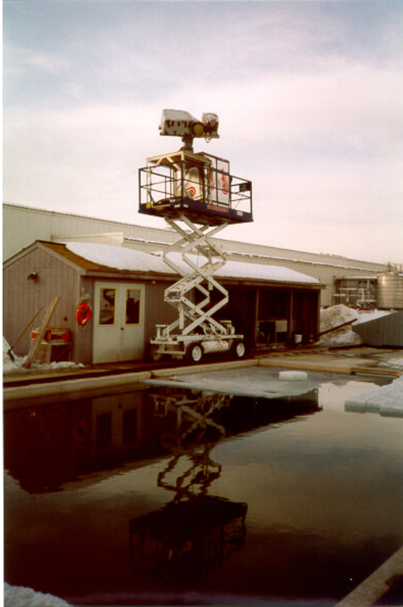
Figure 3. The polarimetric radiometers calibrating, with calm water as a source prior to the growth of the new ice sheet.
