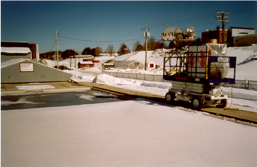
Figure 1. The 37 and 10 GHz radiometers, mounted on the hydraulic lift platform, observing snow covered ice.
