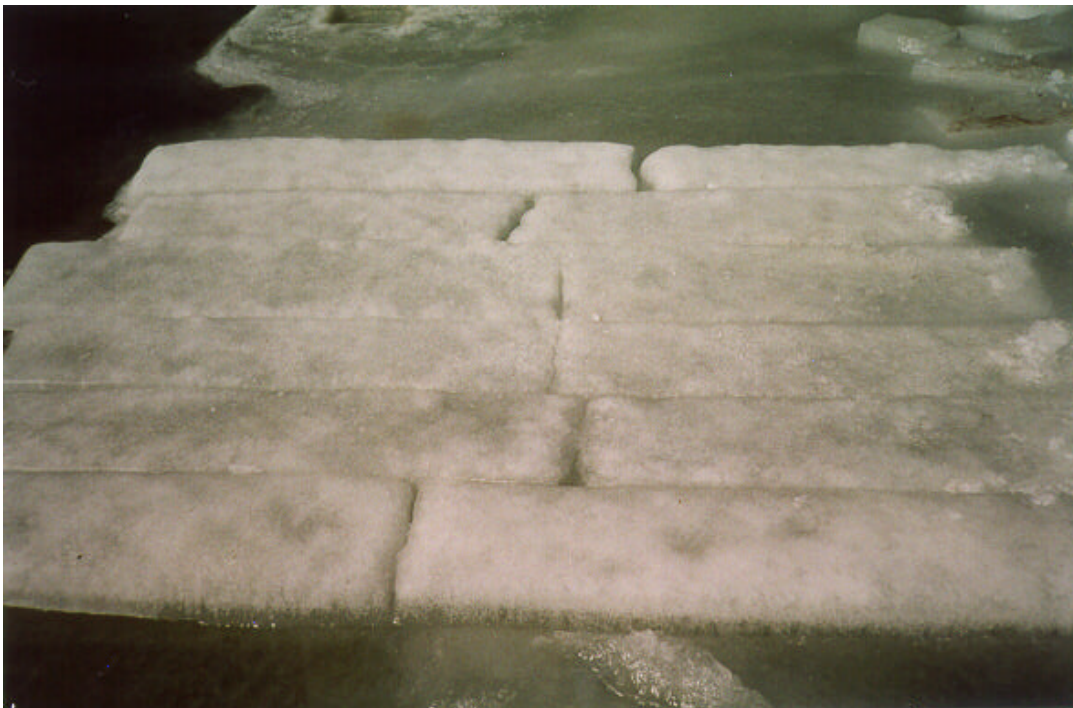
Figure 2. Sections of the ice harvested from the center section of the pond have been placed upon the remaining ice and allowed to desalinate for several days prior to our observations.
