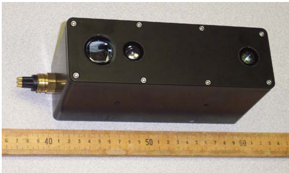
Figure 1. The beta prototype SAM, compatible with AUVs including the Slocum glider. For deployment on the glider, the sensor face is removed from the housing and then seated into the glider payload compartment.
