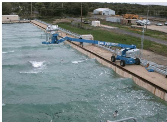
Figure 3: Overview photograph of the OHMSETT wave basin showing the radiometers, mounting crane, and breaking waves generated on the shoal. The shoal is visible in the photograph as the dark shadow behind the breaking wave in the center of the tank.
