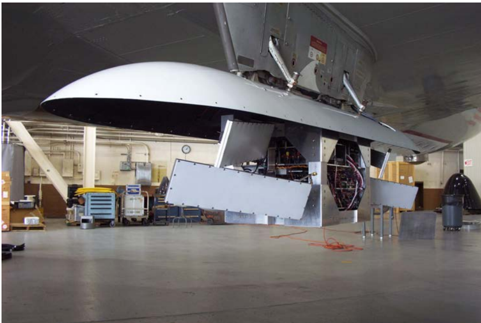
Figure 2: DBI instrument frame and pod top mounted on the NOAA WP-3D wing (pod shell not shown).
