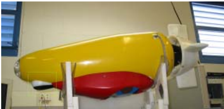
Figure 5. Dual Purpose Acoustic Modem (DPAM) in USBL Configuration mounted on FAU-Squid II
