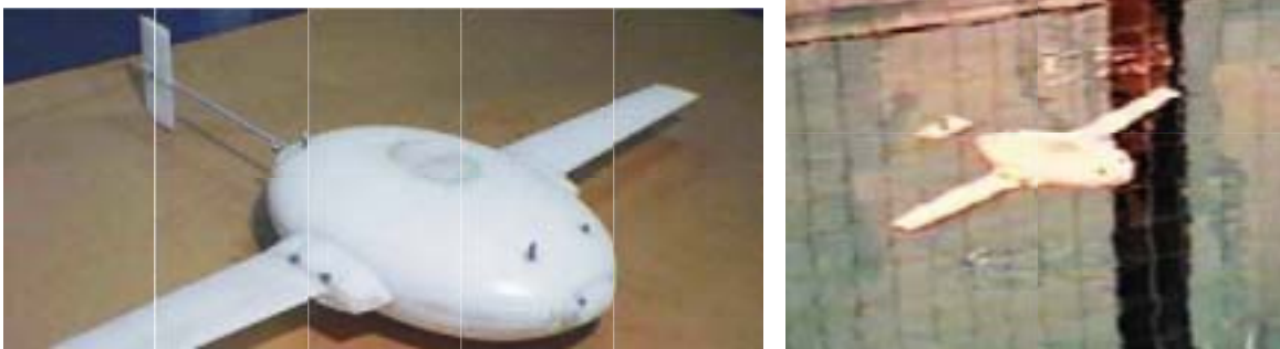
Figure 1: The Princeton laboratory-scale underwater glider, ROGUE. The hull is 18 inches long.
