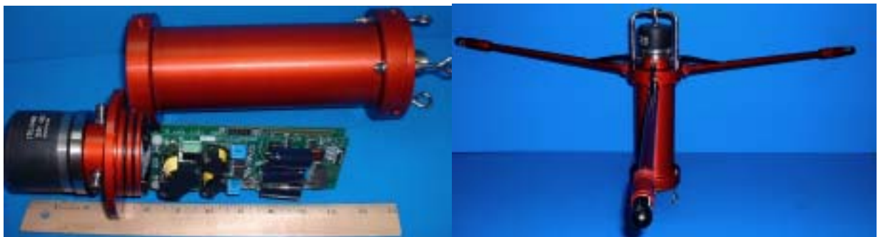
Figure 3. Dual Purpose Acoustic Modem (DPAM) for Communication and Navigation
