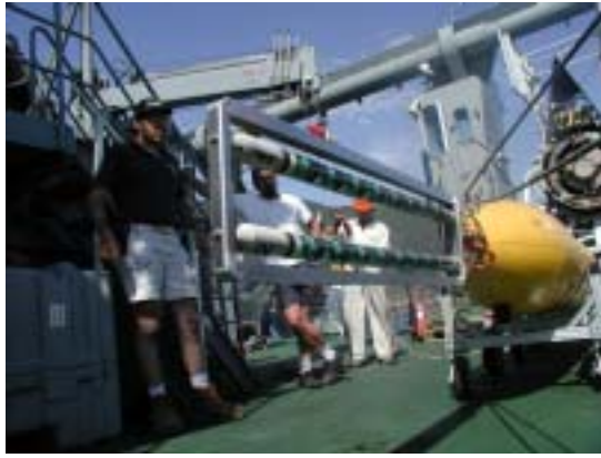
Figure 4. Low-frequency SAS sonar with nose-mounted 2x8 element array and acquisition payload with 4-20 kHz SBP source and 16-channel DSP acquisition system.
