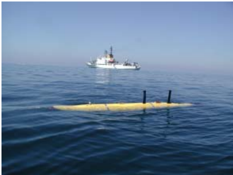
Figure 1: MASAI-02: Caribou Odyssey III AUV ready for launch, with R/V Alliance in background
