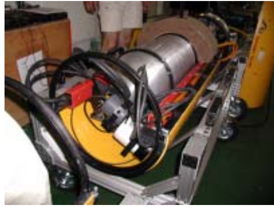
Figure 4. Low-frequency SAS sonar with nose-mounted 2x8 element array and acquisition payload with 4-20 kHz SBP source and 16-channel DSP acquisition system.
