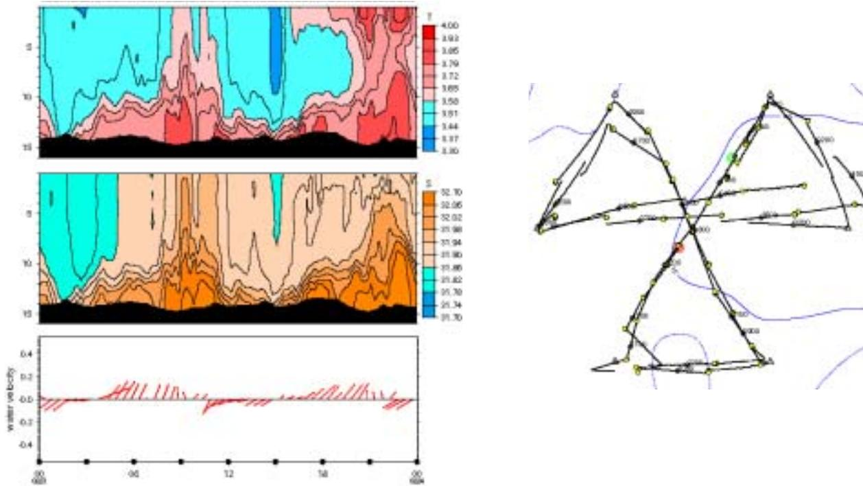
***Above: Temperature and salinity data (time vs. depth) and inferred water velocity during a 24-hour period in Buzzard's Bay. Right panel depicts trajectory of vehicle during the same time period. Water depth was approximately 15 m. Total distance covered in 24 hours was approximately 36 km. Note the +/- 20 cm/s velocity tidal cycle measured by the glider and the corresponding temperature and salinity features.***
