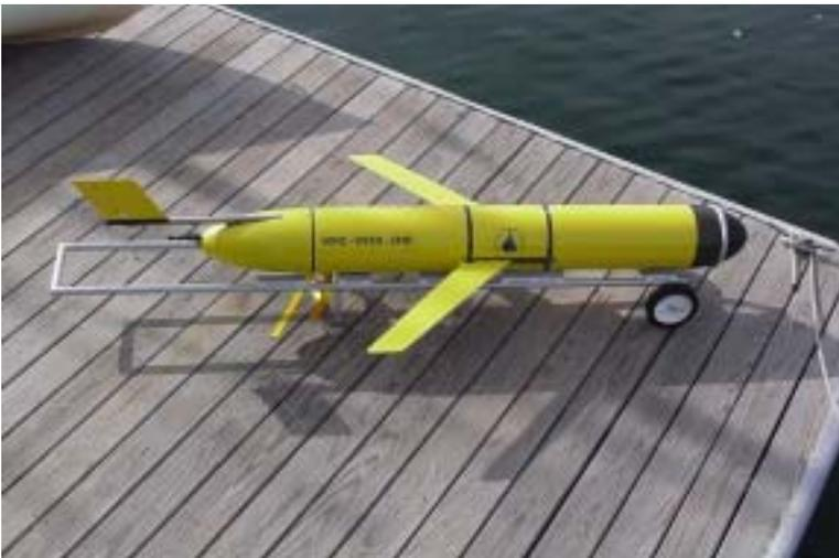
***Left.** Electrically-powered glider ashore and in the water with tail elevated for data transmission.*
