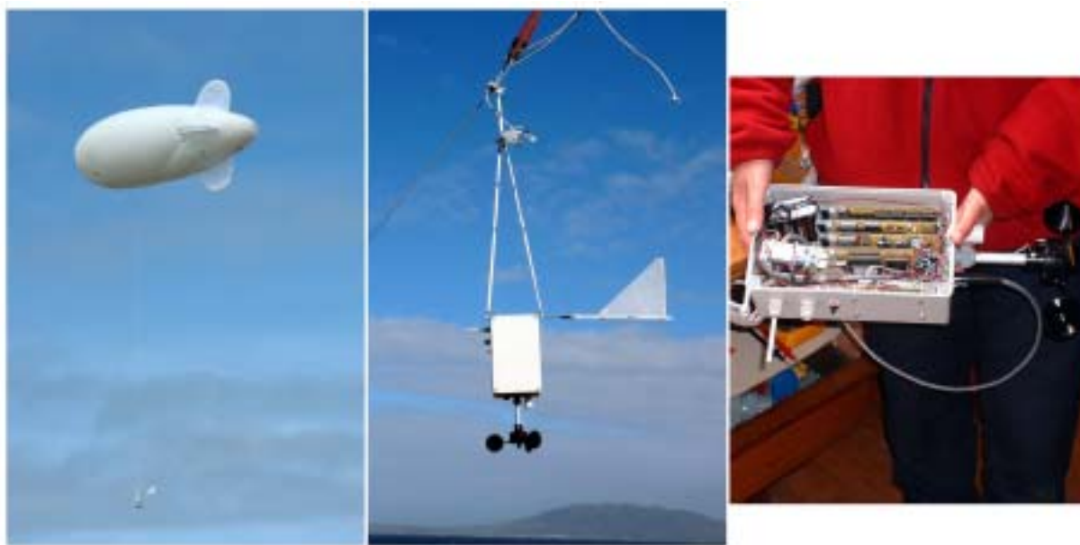
Fig. 1: The prototype optical particle counter sonde operated on a helium balloon and opened to show its components —scatter cell, small pump and data acquisition system.
