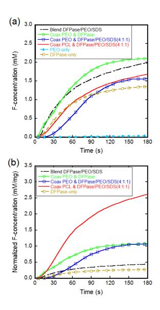
Fig. 6 Enzymatic activity for detoxifying DFP agent through reaction with DFPase: (a) released F concentration vs. time; (b) released F concentration normalized to amount of initial enzyme incorporation vs. time.
