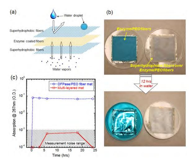
Fig. 10 Multi-layer fiber mat with outer superhydrophobic fibers and inner enzyme containing fibers: (a) schematic of multi-layer fiber mat; (b) demonstration of multi-layer protection of enzyme containing fibers; (c) absorption spectrum (peak wavelength ~ 267 nm) comparison between enzyme/PEO fiber mat and multi-layer fiber mat.
