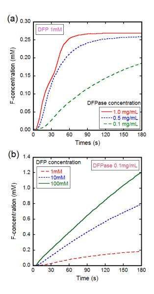
Fig. 8 Reaction kinetics: (a) DFPase concentration effect at 1 mM DFP; (b) linear kinetics at different DFP concentrations with 0.1 mg/mL DFPase concentration.
