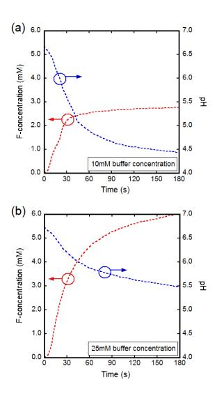
Fig. 7 Dependence of DFP-DFPase reactions on pH change in solution: 2.5 mg of DFPase added in 10 mL of PIPES buffered DFP solution made of 3 mL of 25 mM DFP solution and 7 mL of (a) 10 mM or (b) 25 mM PIPES buffer solution). Measurement repeated by 3 times and averaged graphs are shown.
