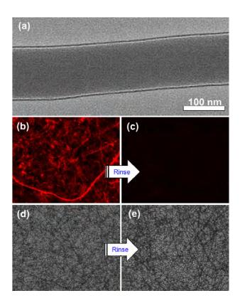
Fig. 3 Core-sheath structure observation using (a) TEM; and Fluorescence microscopy of coaxial fibers containing Keystone Red dye in the sheath, before and after rinsing with water: (b) initial dark-field image (c) dark-field image post-washing; (d) initial bright-field image (e) bright-field image post-washing. Exposure times for bright-field and dark-field modes are 2 ms and 2 s, respectively.
