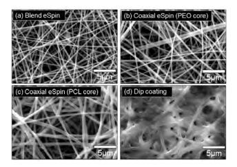
Fig. 4 SEM observations of electrospun fibers (a) PEO & DFPase blend fibers with 1:1 wt. ratio; coaxial fibers with DFPase sheath and (b) PEO core / (c) PCL core; (d) PCL fibers dip coated with DFPase solution.
