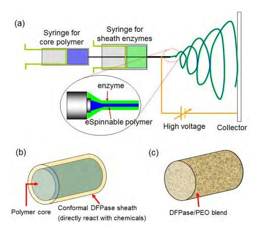
Fig. 2 Electrospinning of enzyme containing fibers: (a) coaxial dual solution electrospinning; (b) core-sheath coaxial fiber with polymer core and conformal DFPase containing sheath; (c) uniform DFPase/PEO blended fiber using single solution electrospinning.
