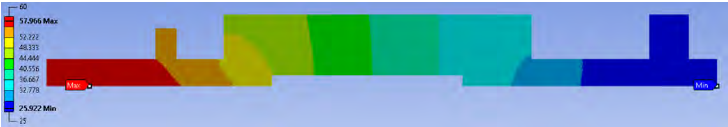
Figure 12. Contours of Temperature throughout casing for 90% speed.
