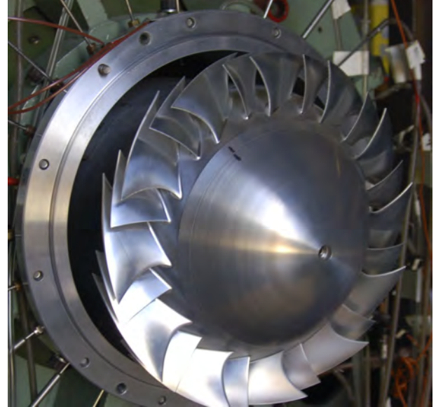
Figure 2. Transonic Splitted Rotor without casing.
