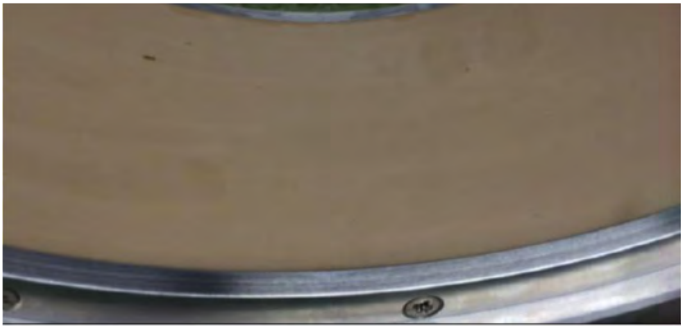
Figure 5. Photo of inside of casing just above the rotor showing the pre-machined abradable material considered to be adiabatic.
