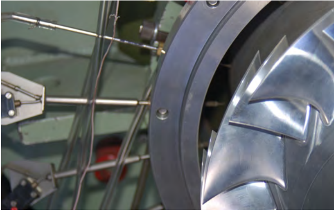
Figure 4. View of rotor showing combination probes.
