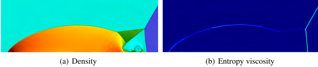
Figure 3: Double Mach reflection, t = 0.2 , \mathbb{P}_1 approximation.
