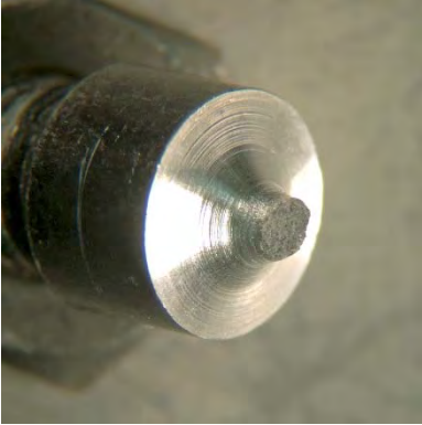
Figure 11. Typical ductile fracture surface resulting from a screw tensile strength test.
