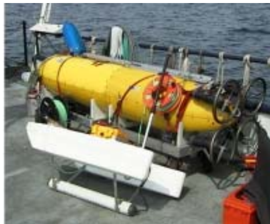
Figure 1. ROVEX with ROBOT payload [The Laser imaging sensor ROBOT as an AUV payload connected to the autonomously guided underwater vehicle ROVEX. The white surface communications tow float is shown in the foreground.]
