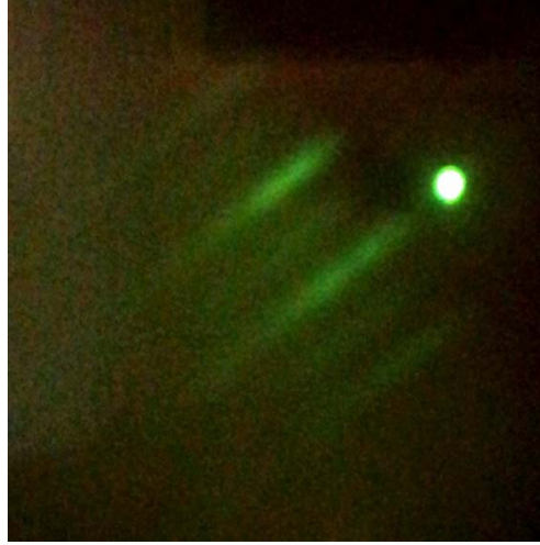
Figure 5.3. 2x2 RHEED reconstruction during the cool down process after growth
