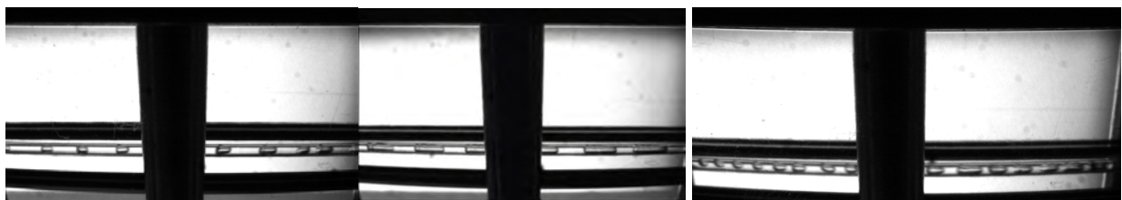
Fig.3.9 Samples of slug flows recorded by the camera located far downstream corresponding to three different experiments at 0g.
